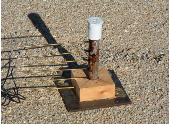
Figure 9. AFRL Modified Rate Stick Test Configuration
